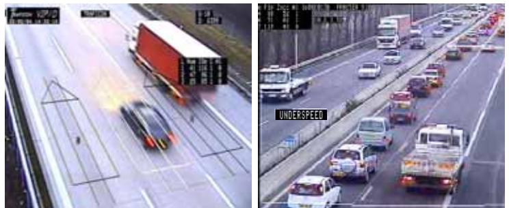
Sudden speed variations are detected within seconds to help preventing secondary accidents.
