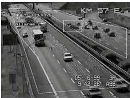
The system offers both alarm text & position indication.
