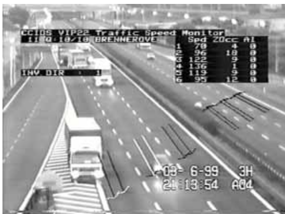
The truck backs up to the exit and causes an alarm (INV DIR:1).
