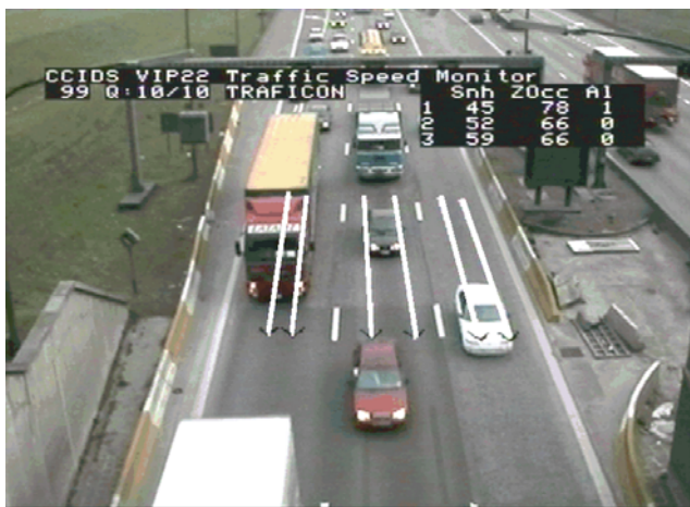
Line following principle for speed measurement with video detection.
